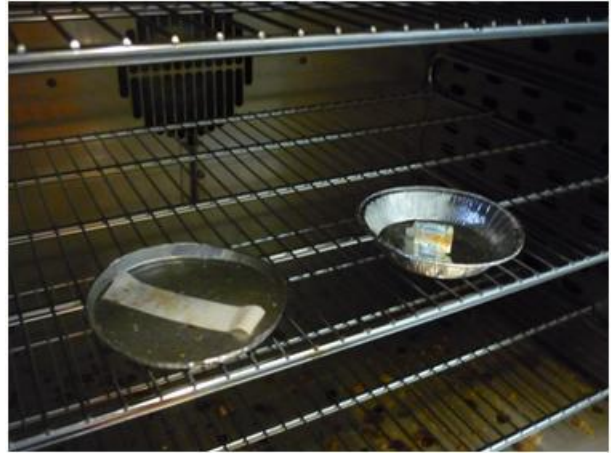
Photo 4: Dry sample for 2 hours at 80°C (W1)
