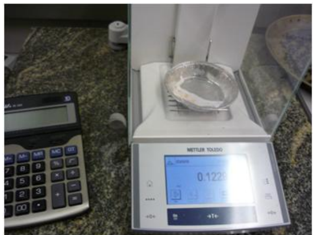
Photo 5: Analytical balance to weigh sample after washing (W3)
